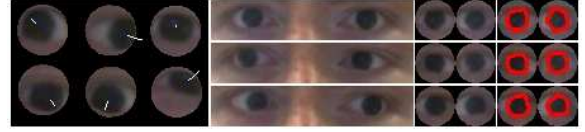
Fig. 10. (First column) 3D rendered eyeballs with white lines indicating optical gaze direction; (second column) original 2D image used for 3D iris detection; (third column) 3D eyeballs rendered with the iris looking into the camera; (fourth column) iris contours, shown as red dots between the iris and the rest of the eyeball, found on rendered eyeball image.
