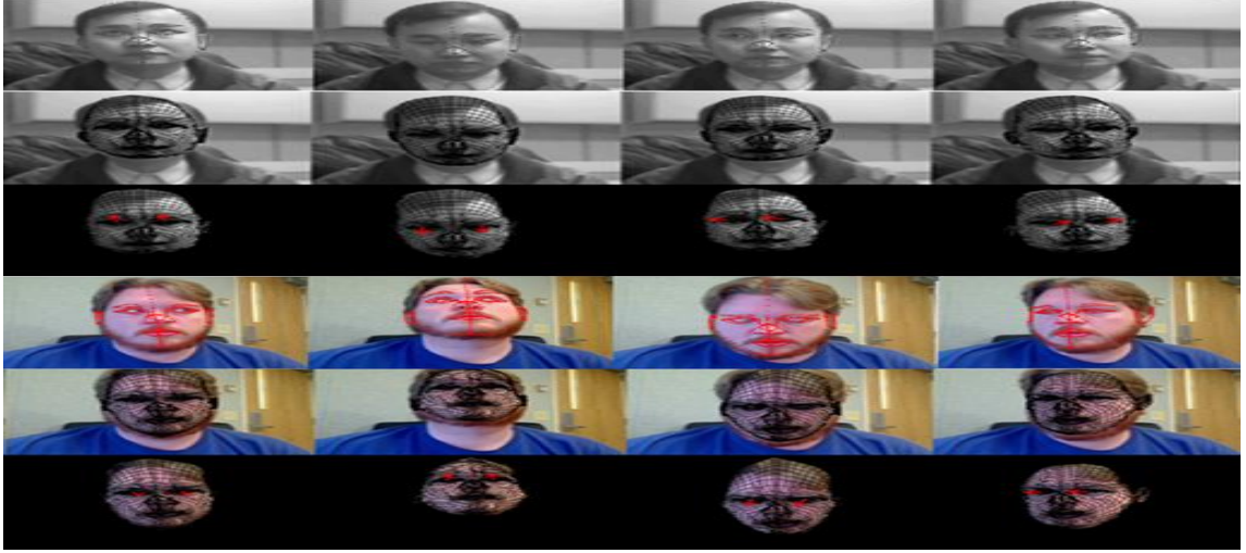
Figure 5. Low-resolution videos for two subjects. Tracked feature points; generated models; and detected eye sight directions(shown as red arrows).
