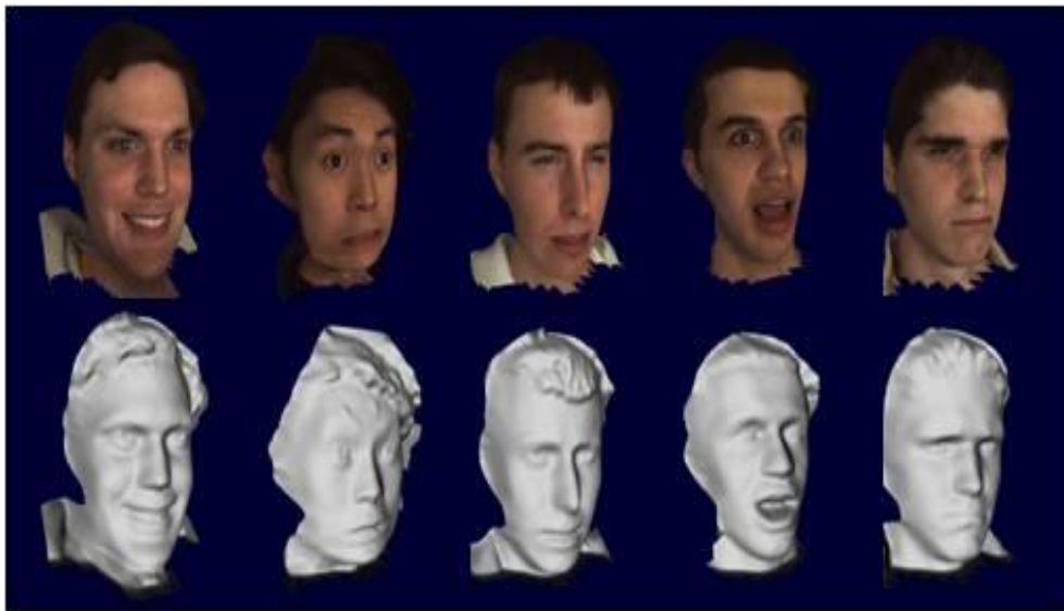
Figure 11. Examples of 3D scans from 4DFE: textured models shown in upper row and shaded models in bottom row
